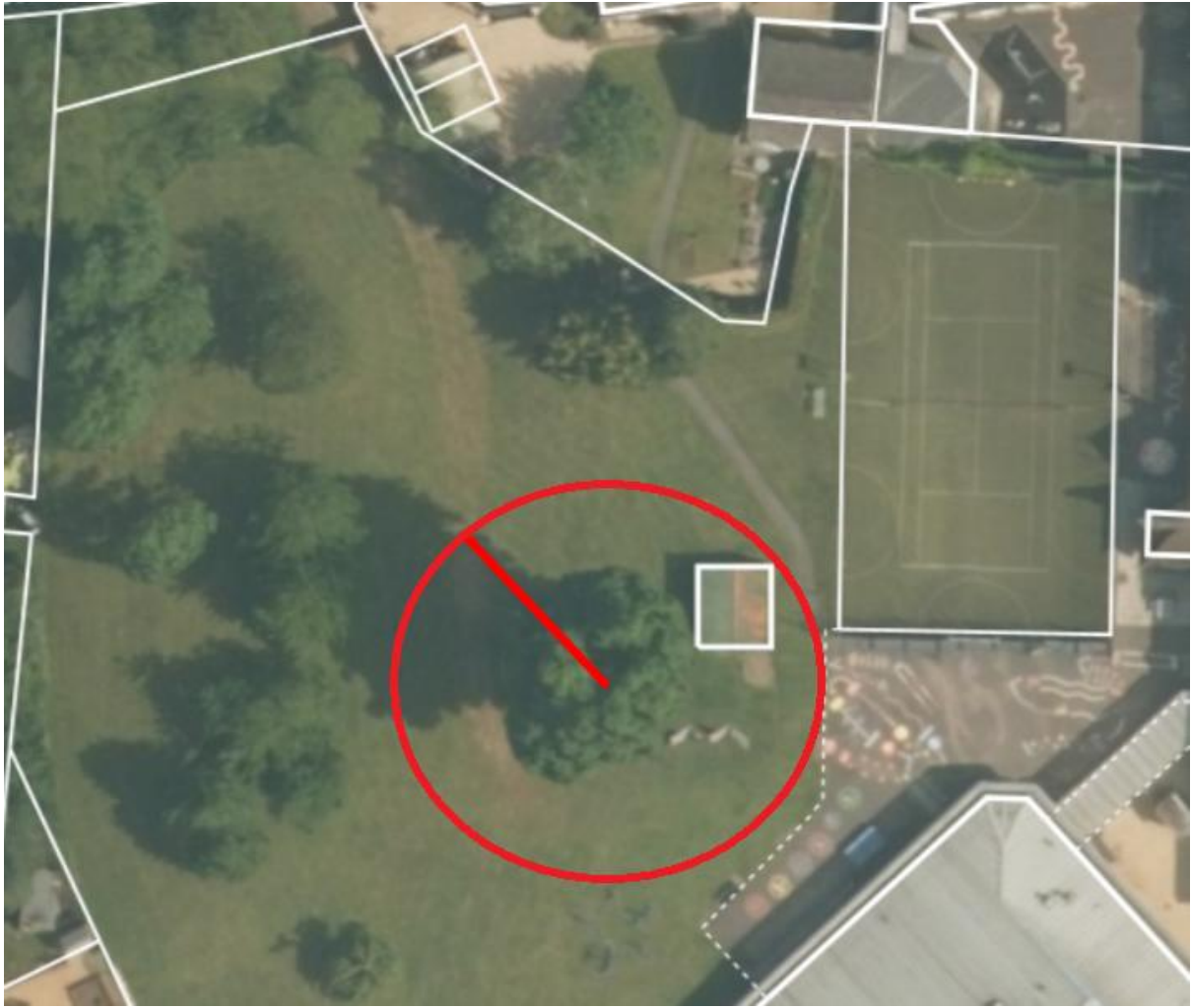
Indicated (approximate) 15m radius from lime tree 3087 and root protection area.
