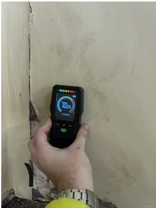
P39 – High readings of moisture however results not accurate due to foil behind paper.
