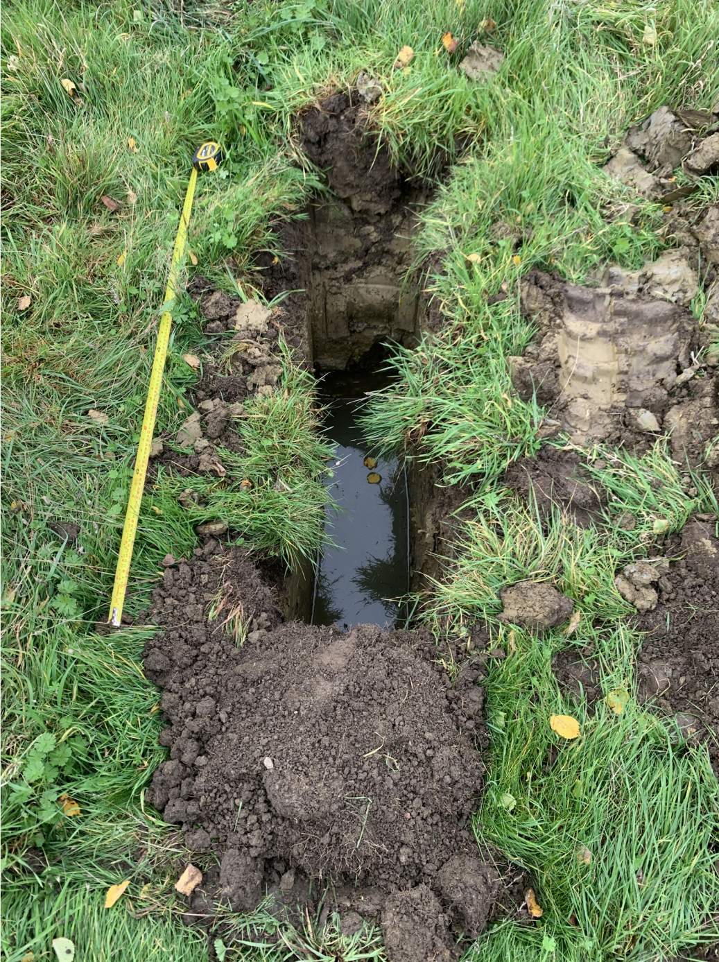
Area 1 – Soakaway Test Trial Hole
