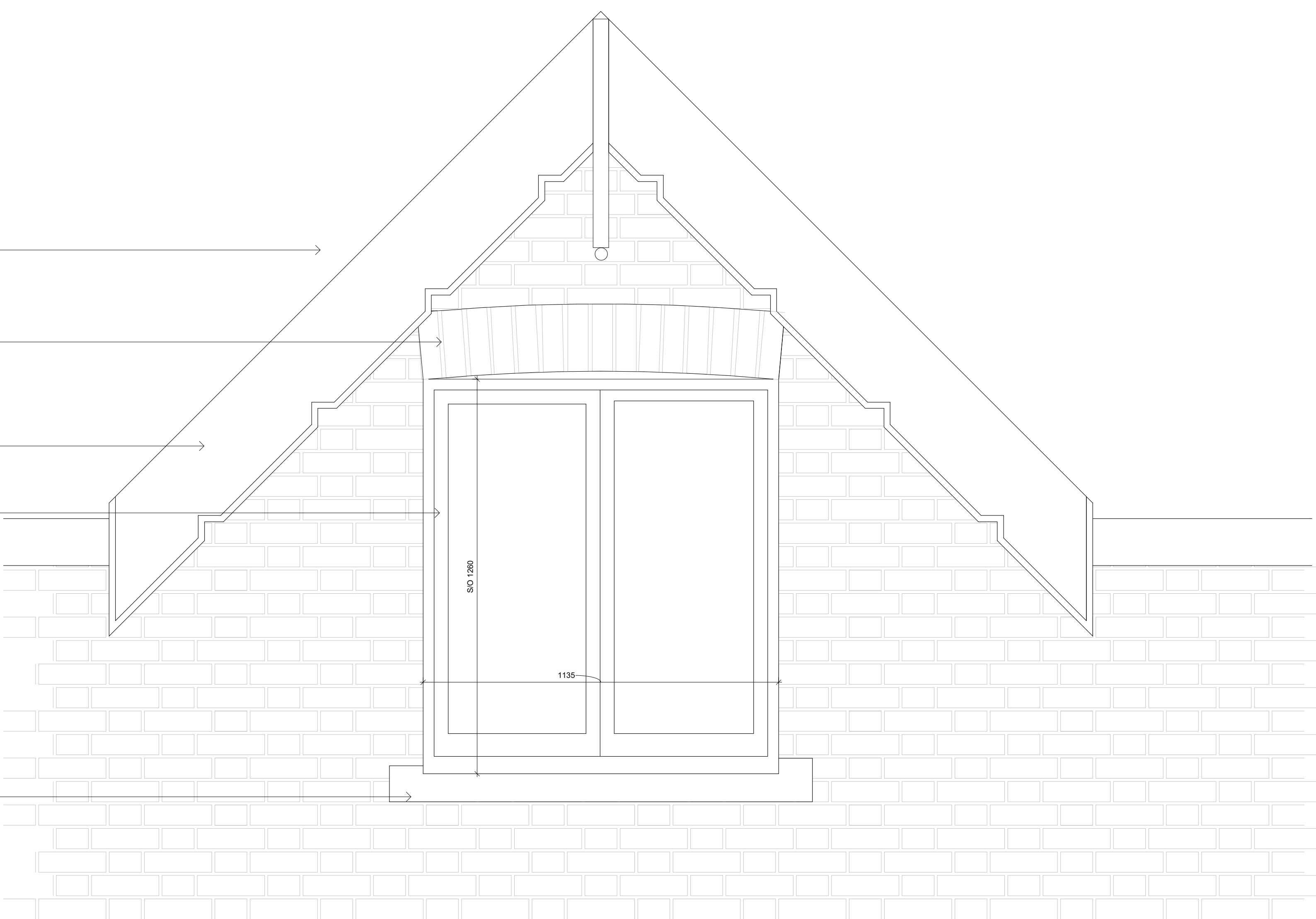
Dormer Window Elevation 1:10
