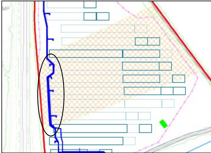
Plate 4: High voltage cable trench within the above-ground foundation zone in Field 12
