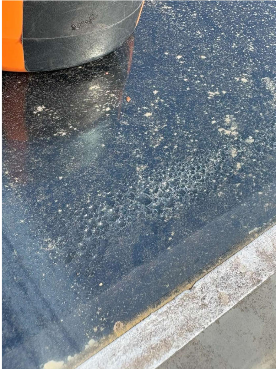
Image 6: Condensation on Glazing Pane.
