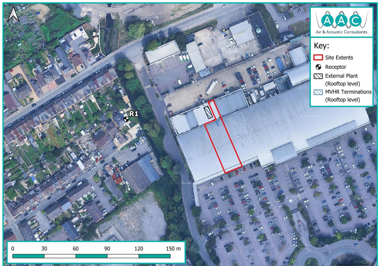
Figure 5.1: Fixed Plant Location
