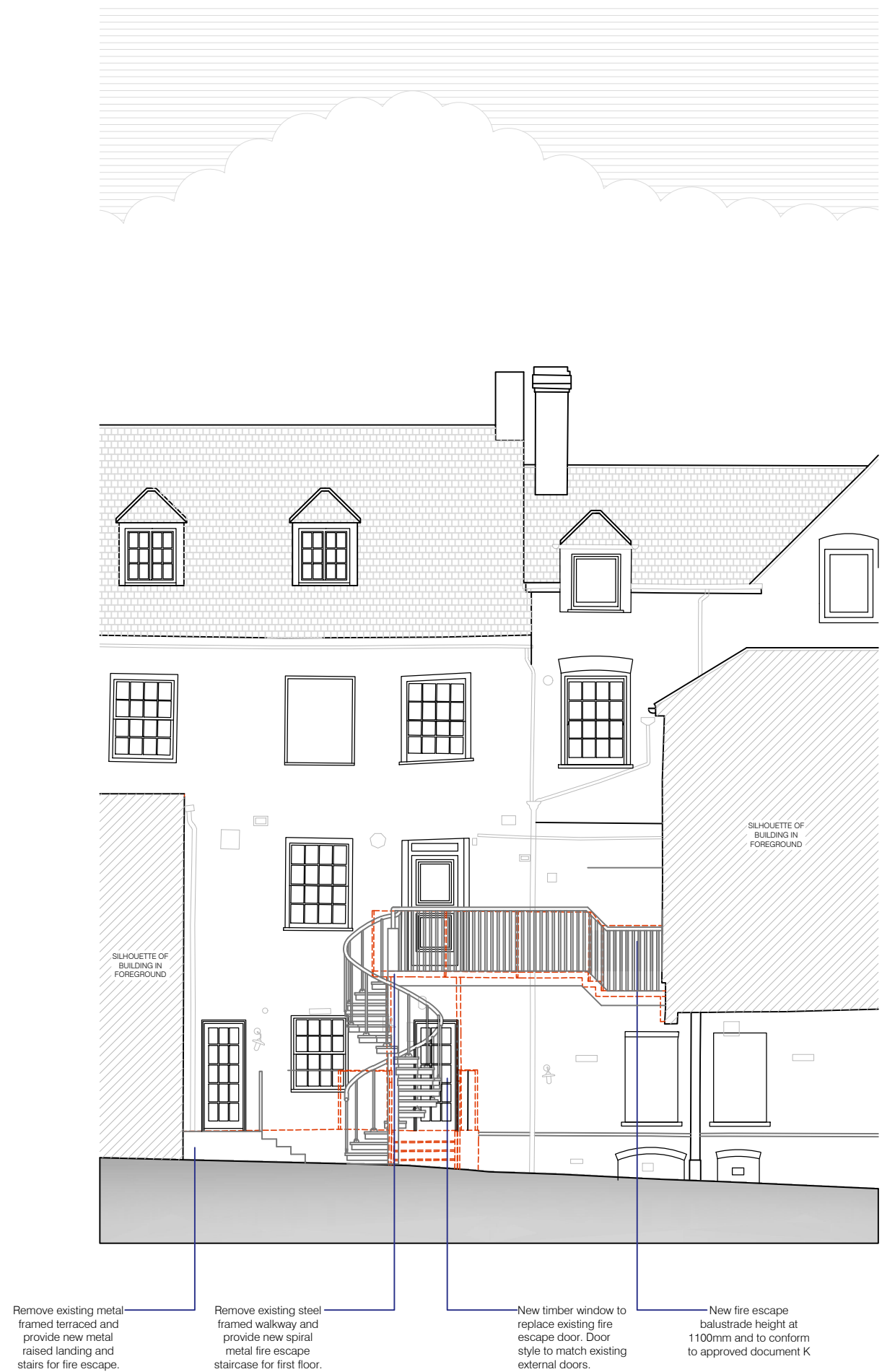
PROPOSED ELEVATION A Scale 1:100
