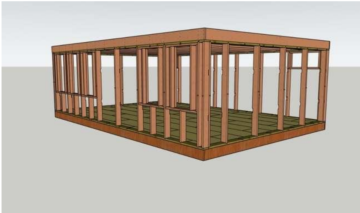
Figure 1- Day 1 Skeleton completed
