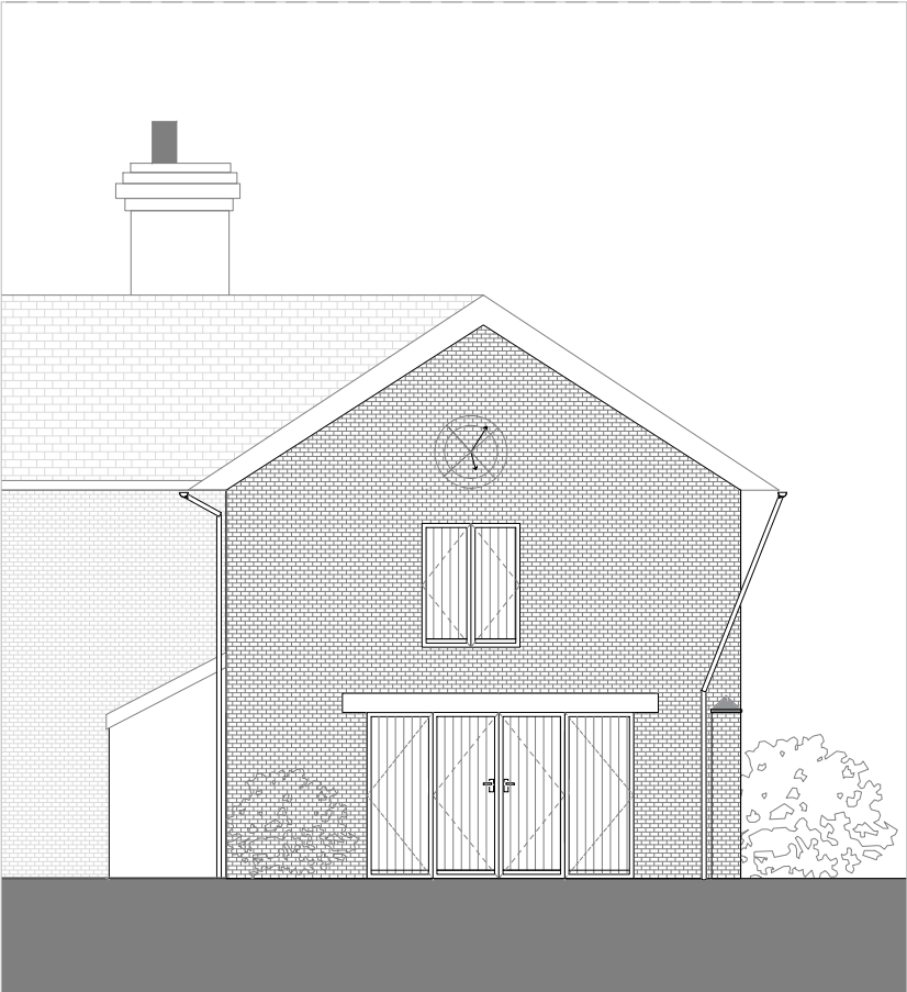
02 - Proposed Front Elevation of barn (South)
