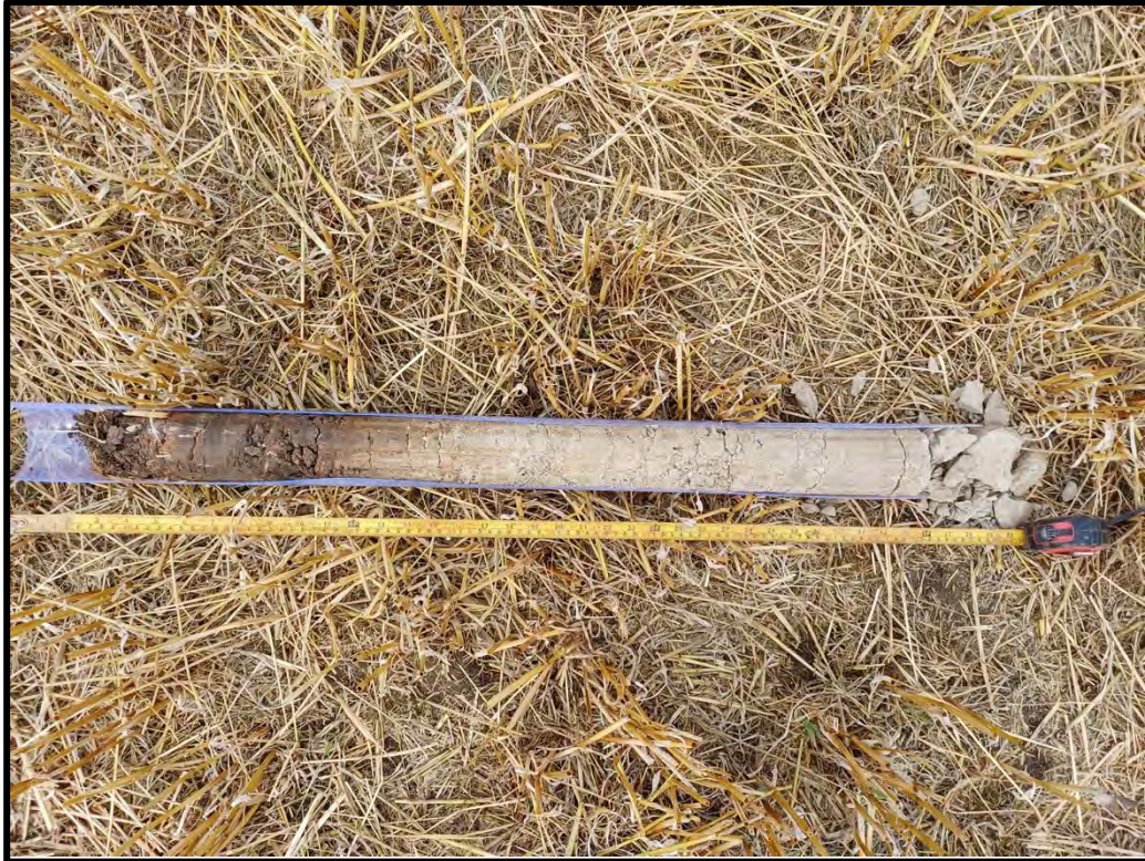
Borehole Core (0.0 – 1.0m)
