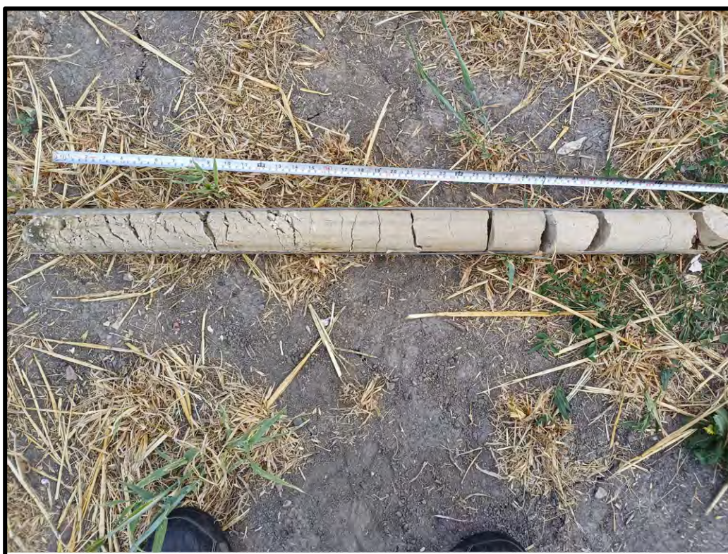
Borehole Core (0.7 – 2.0m)
