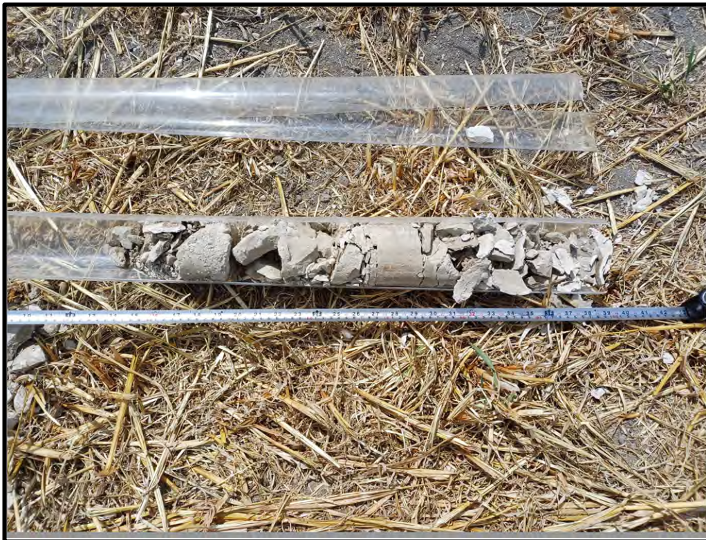
Borehole Core (0.7 – 1.0m)
