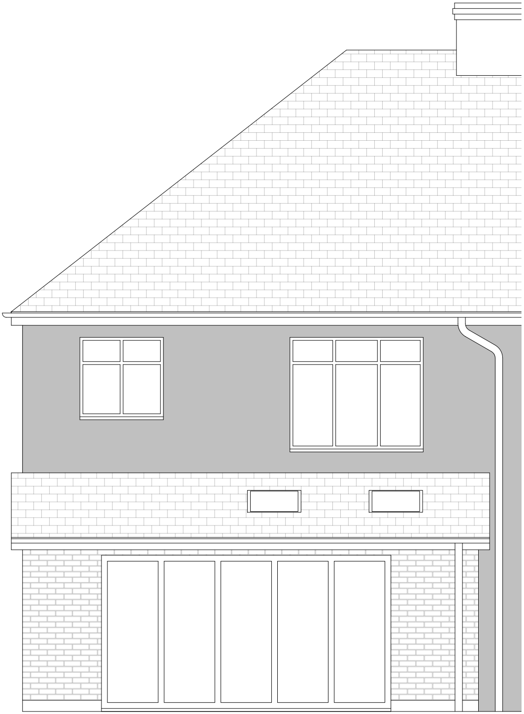
EXISTING REAR (SOUTHERN) ELEVATION (SCALE 1:50)
