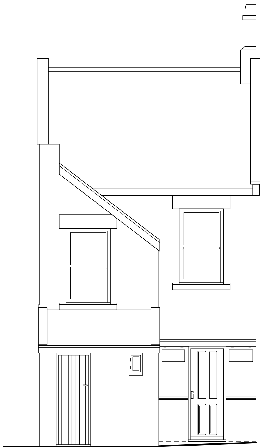
EXISTING REAR ELEVATION
