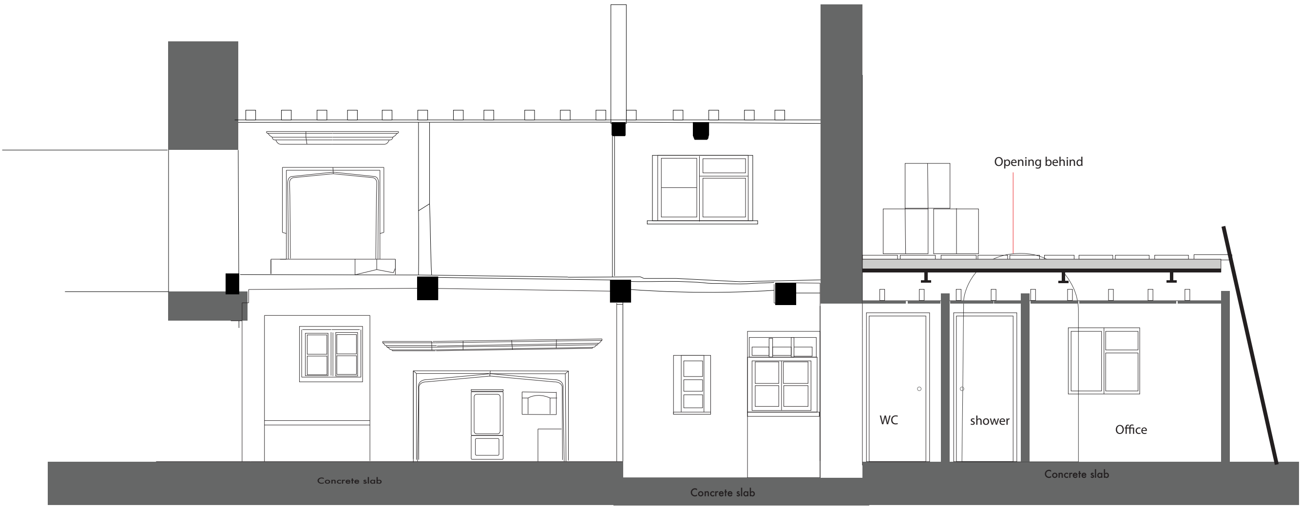
Existing Section A-A Through Farmhouse Scale 1:50@A2
