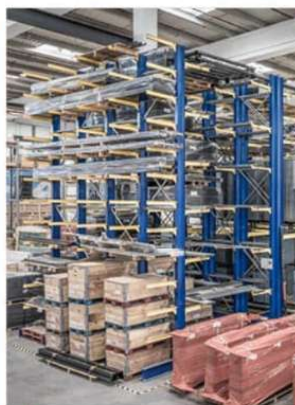
Cantilever FIFO racking system
