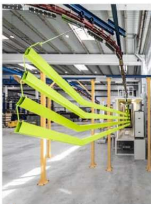
Automated electrostatic painting plant by coating
