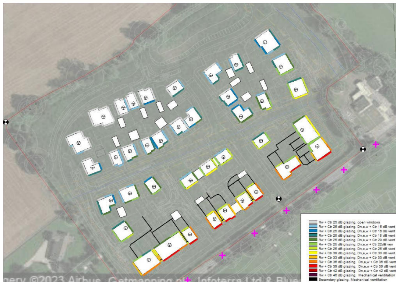
Figure 6: Glazing and Ventilation Strategy – Bedrooms, First Floor
