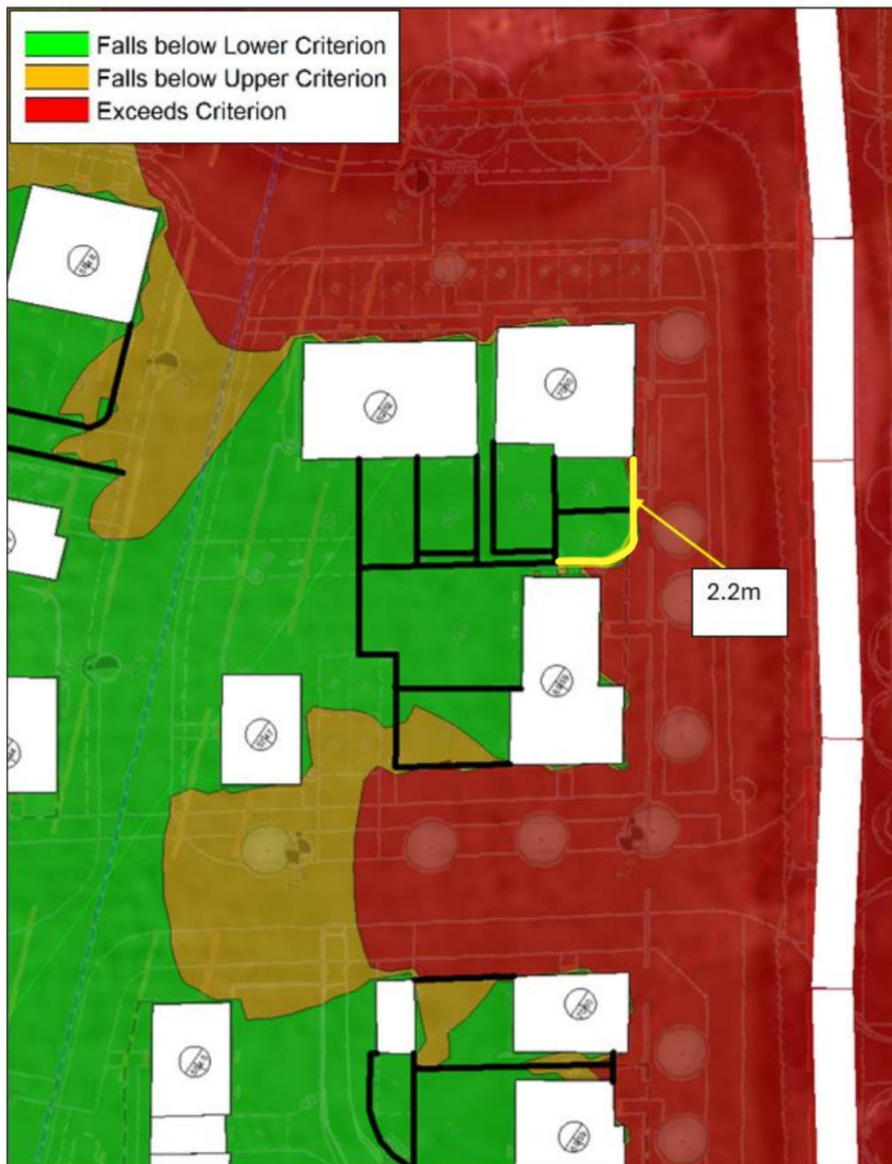
Figure 10: External amenity with 2.2m fence mitigation at plots 47 and 48
