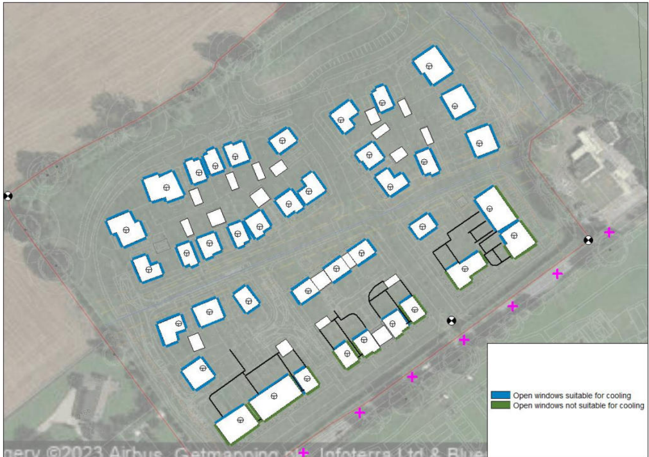
Figure 7: Cooling strategy for overheating scenarios – Ground Floor (bedrooms only)
