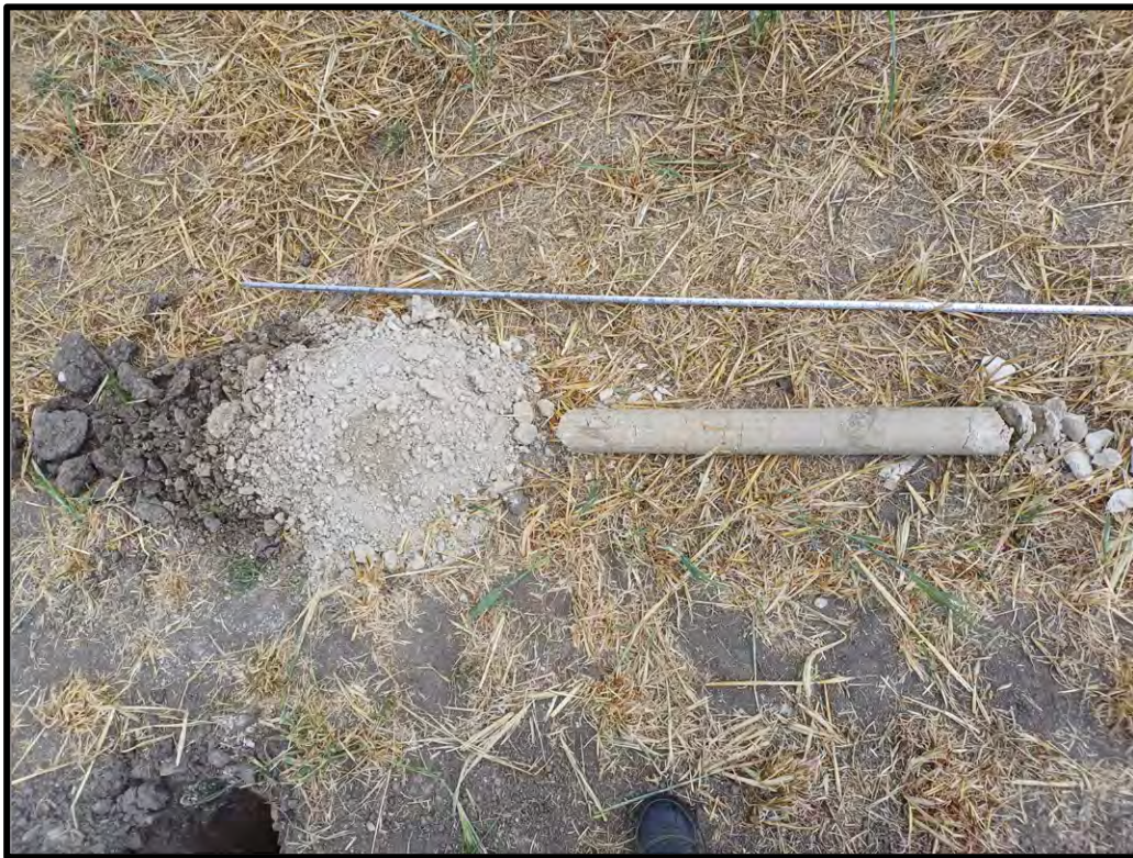
Starter pit arisings (0.0 – 1.0m) and Borehole Core (1.0 – 2.0m)
