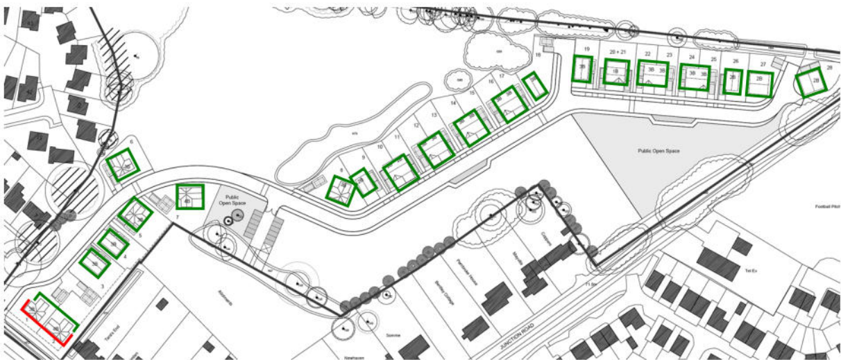
Façade acoustic specification zones (all levels)
