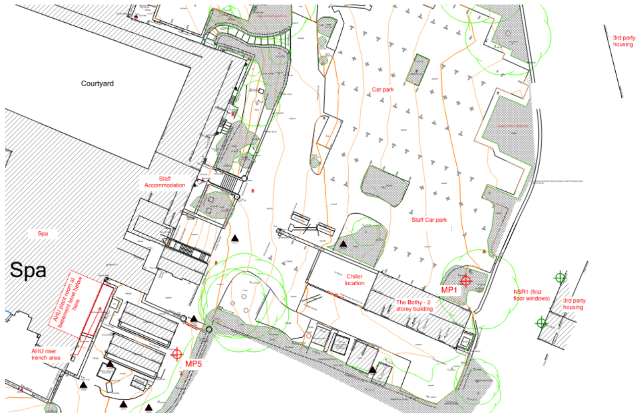
Figure 1: Location plan showing the measurement positions and AHU location.
