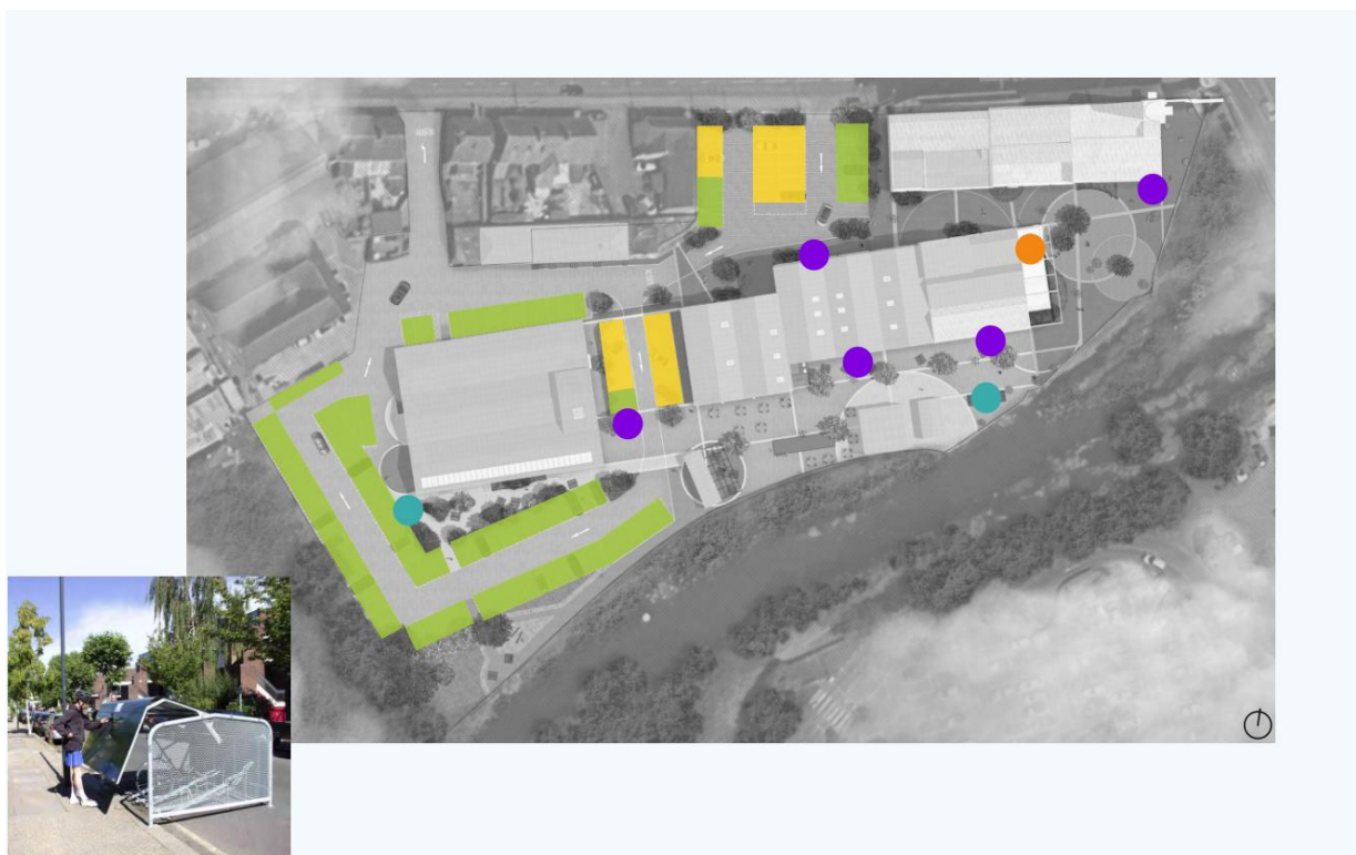
Figure 11: Extract from the Design Note showing the vehicular and cycle parking locations. Yellow are the residential parking spaces and green for business uses. The orange dot is covered and secure residents cycle storage. Turquoise is similar for the business users. Purple dots are for Sheffield stands.
