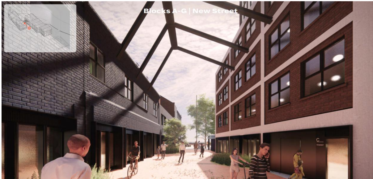
Figure 8: The internal pedestrian space created by demolition between Blocks C and D with steels retained to reflect the historic roofscape, new windows created to the internal elevations which are sympathetic to the existing fenestration whilst retaining a circa 10 metre intervisibility between the new residential units.
