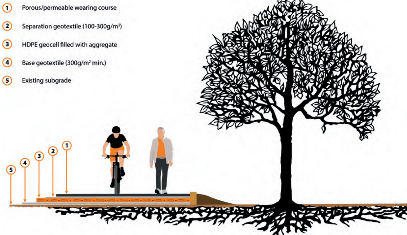
Figure 1: The basic approach to using cellular confinement systems for ground protection near trees [image courtesy of Core LP].
