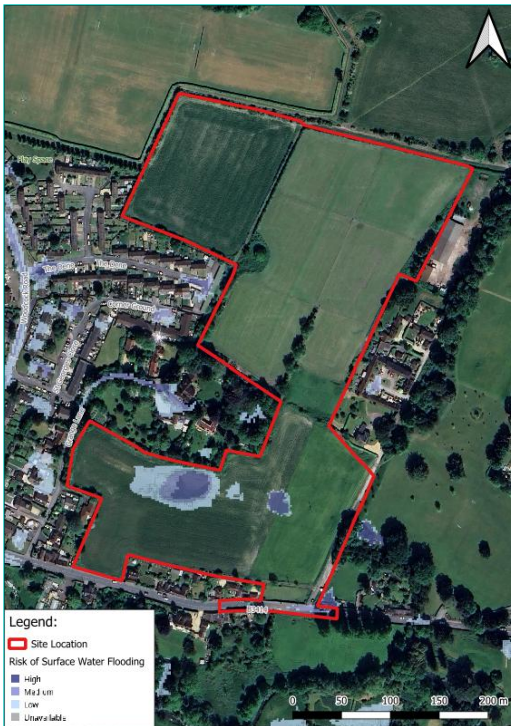
Figure 2: Extent of Surface Water Flooding
