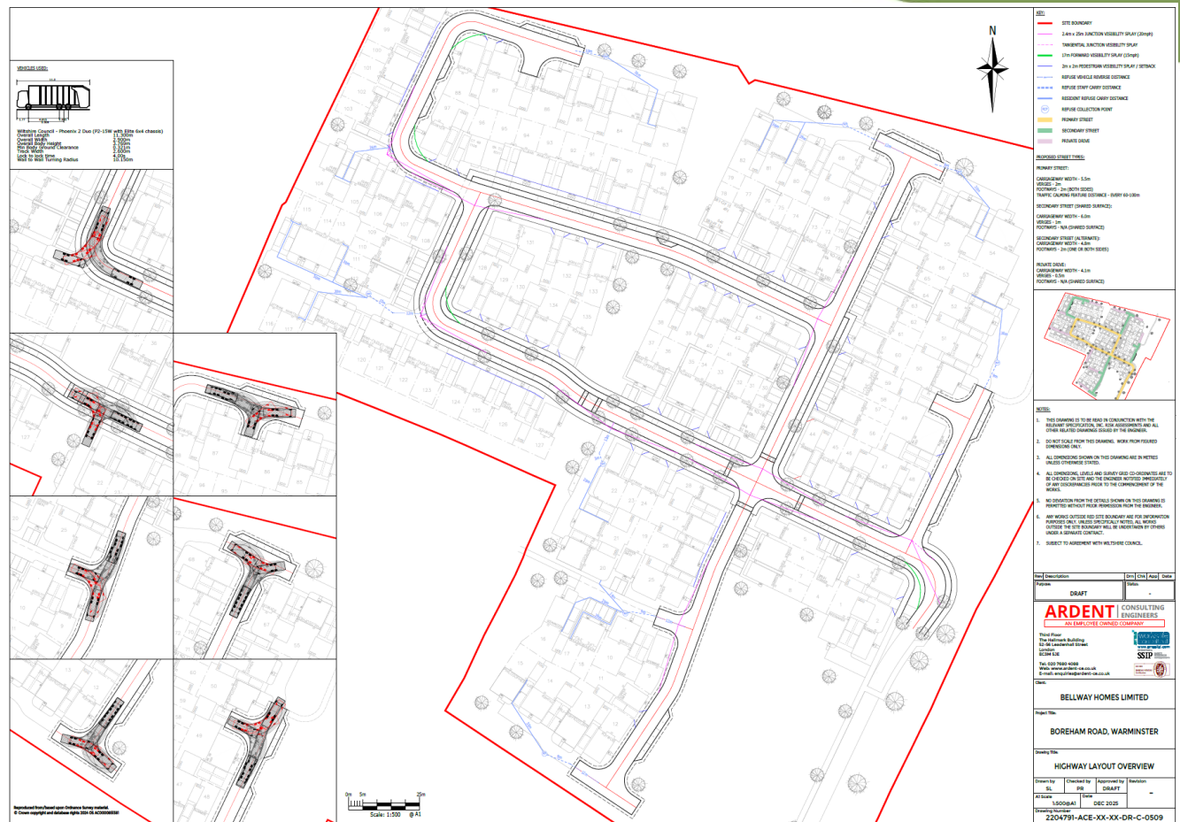
Figure 7 : Refuse vehicle tracking (Source: Ardent Consulting Engineers)
