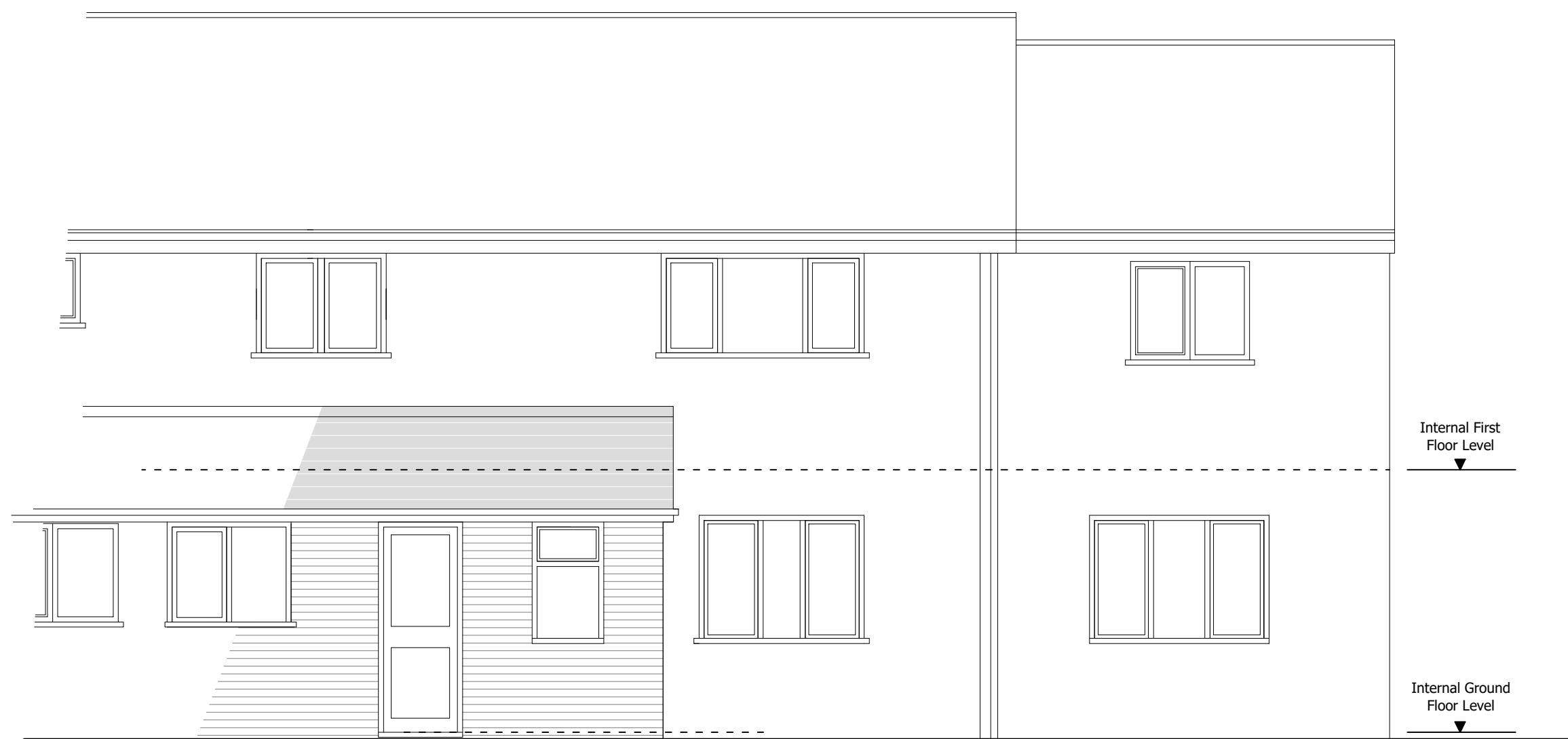
Proposed Elevation Looking South East
