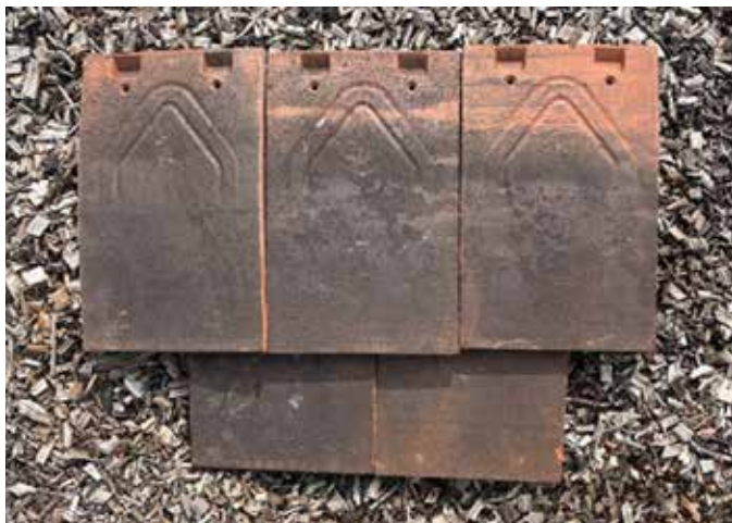
Proposed tiles: Edilians Phalempin Plain Roof Tile, Weathered, 110 to be blended in with existing salvaged clay plain tiles
