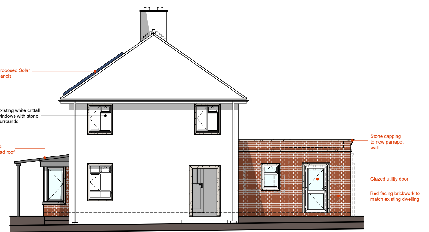
Proposed Side Elevation Scale 1:100
