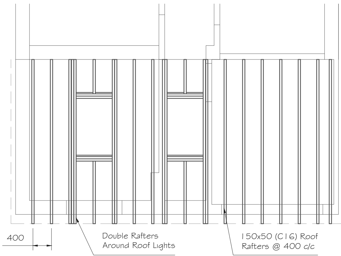
ROOD RAFTER PLAN (FRONT) Scale 1:50
