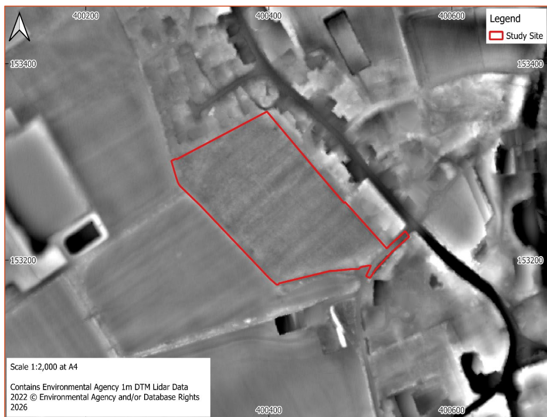
Plate 6 1m DTM LiDAR data for Study site rendered using simplified local relief model analysis
