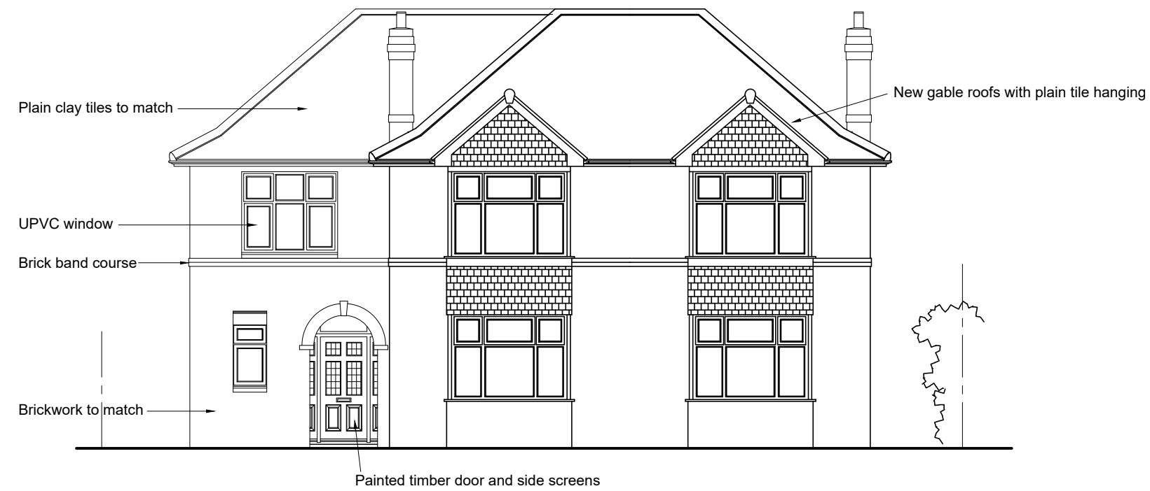
SOUTH EAST (front) PROPOSED ELEVATIONS scale 1:100
