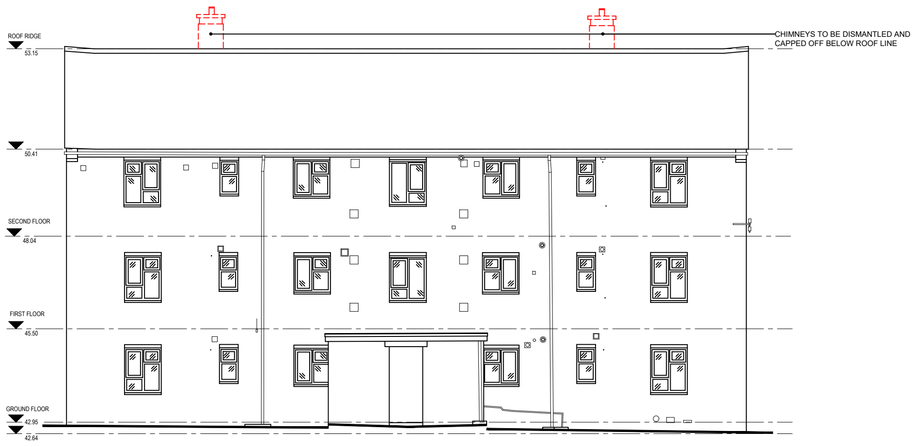
3 EXISTING - NORTH EAST ELEVATION A/003 SCALE 1:100
