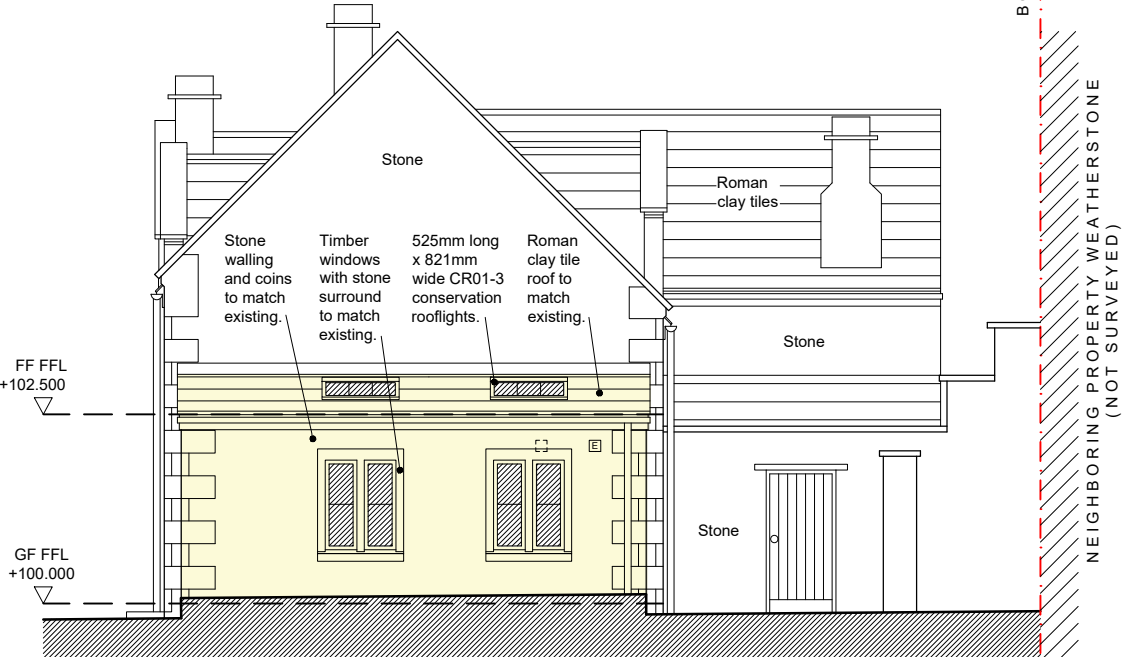
Proposed North Elevation
