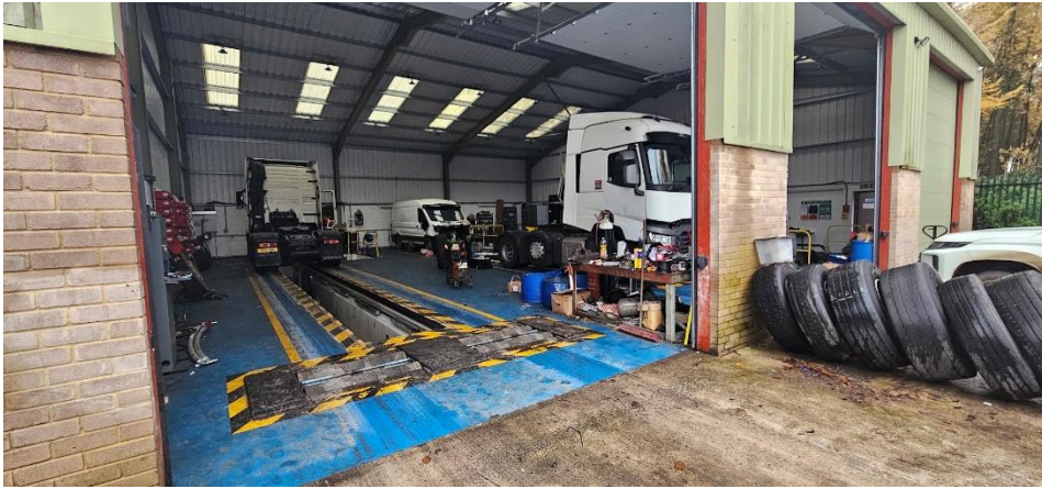
Above: Inside workshop building, showing the requirement for the extra building height, for accommodating HGV's and other tall vehicles whilst they are being repaired/ serviced
