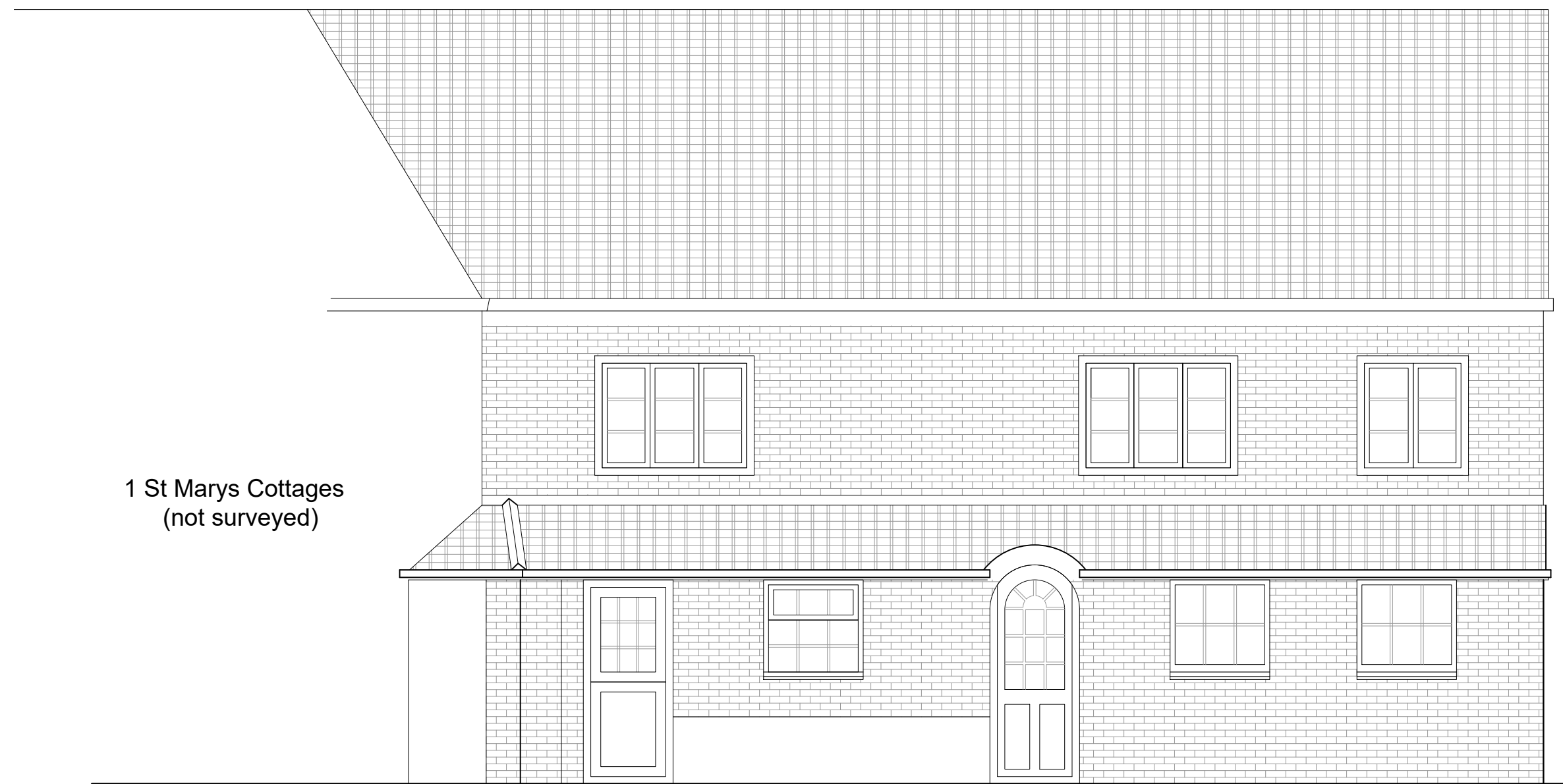
EXISTING WEST FACING ELEVATION (partial) Scale 1:50
