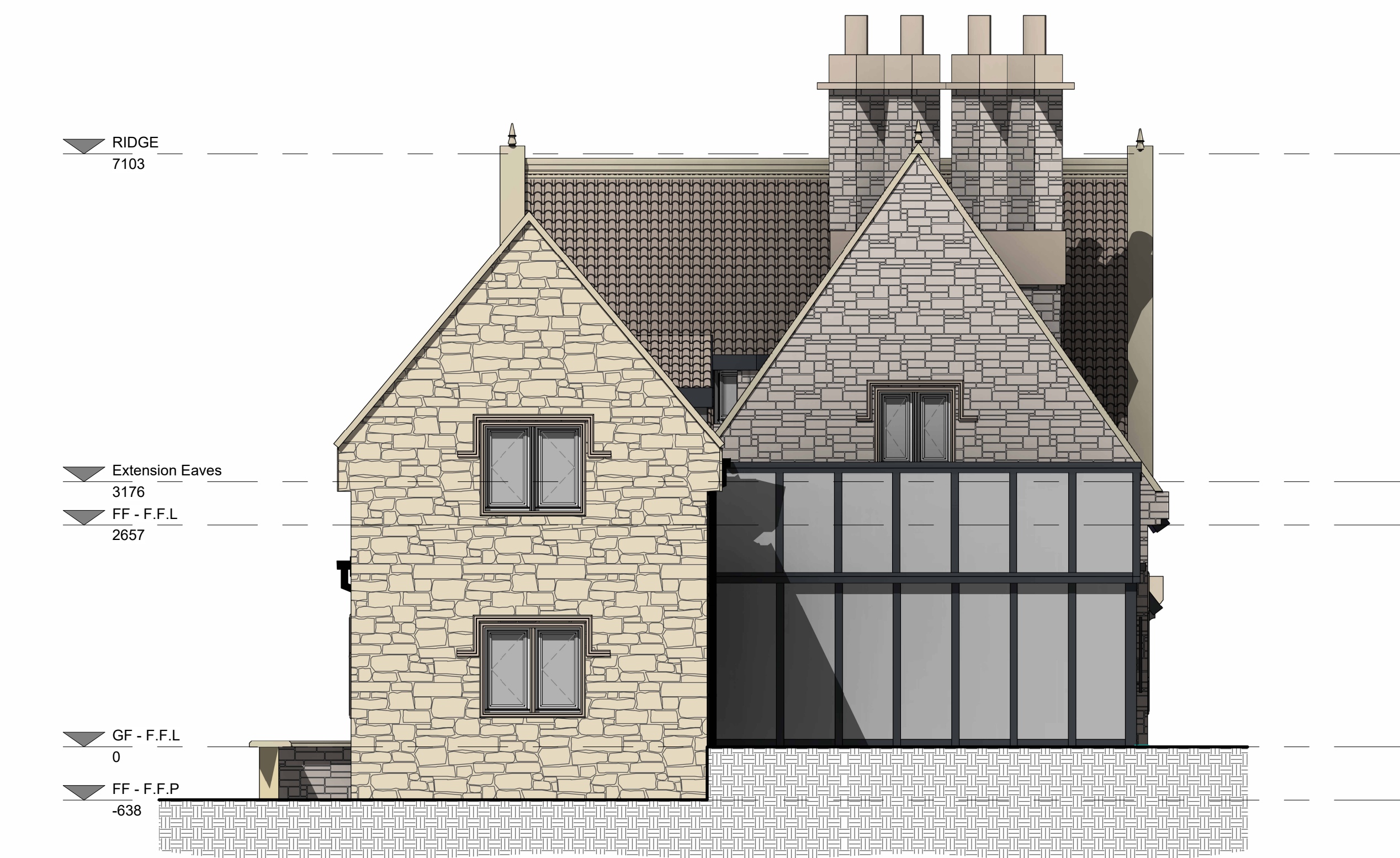
3 EXT_Rear Elevation - Materials 1 : 50
