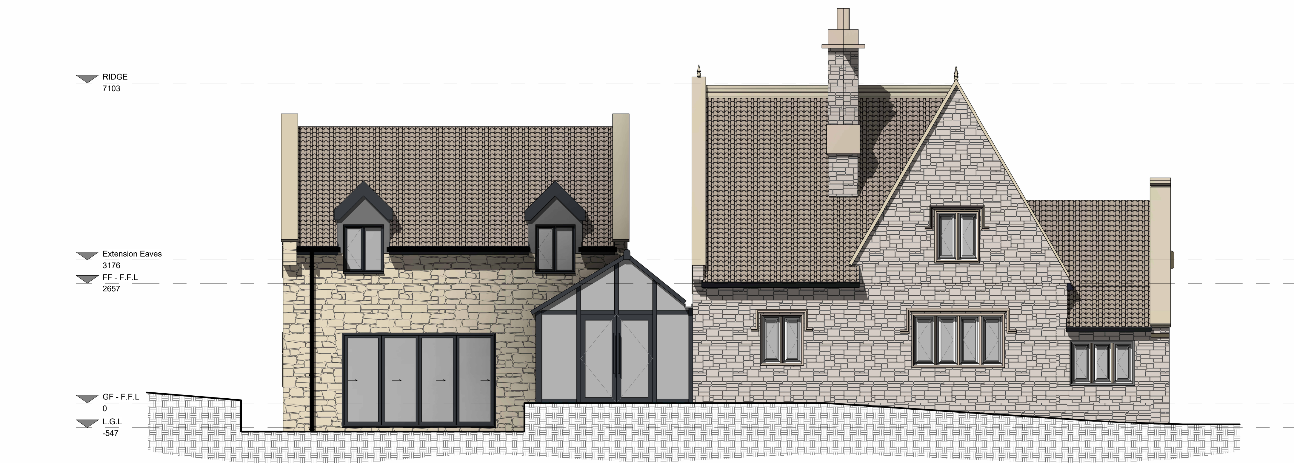
4 EXT_Side Elevation_02 - Materials 1 : 50
