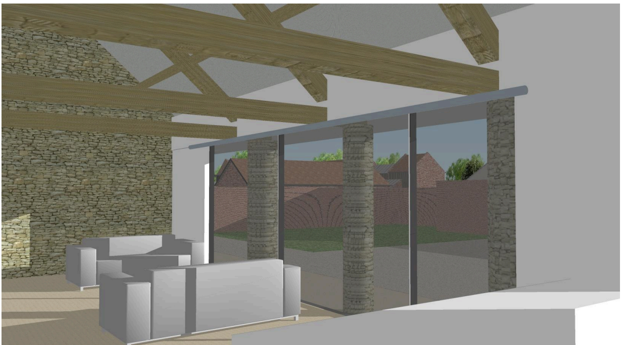
3.03 Fig 3. The current permission within the building shows an unbalanced roof structure. It also leads to the external stone piers being a collection for cobwebs, and dirt between the window and the stone pillars. Under the current permission, it will be necessary to install further timbers to support either curtains or blinds so they will be set further back into the building, again separating the structure in an awkward manner. At the time when the original permission was granted it was not known that the intermittent piers were a different diameter.
