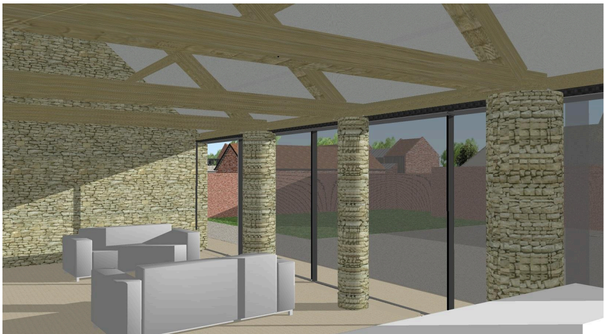
Fig 5. Image showing the trusses sitting on the stone columns that are no longer hidden, true to the original built form
