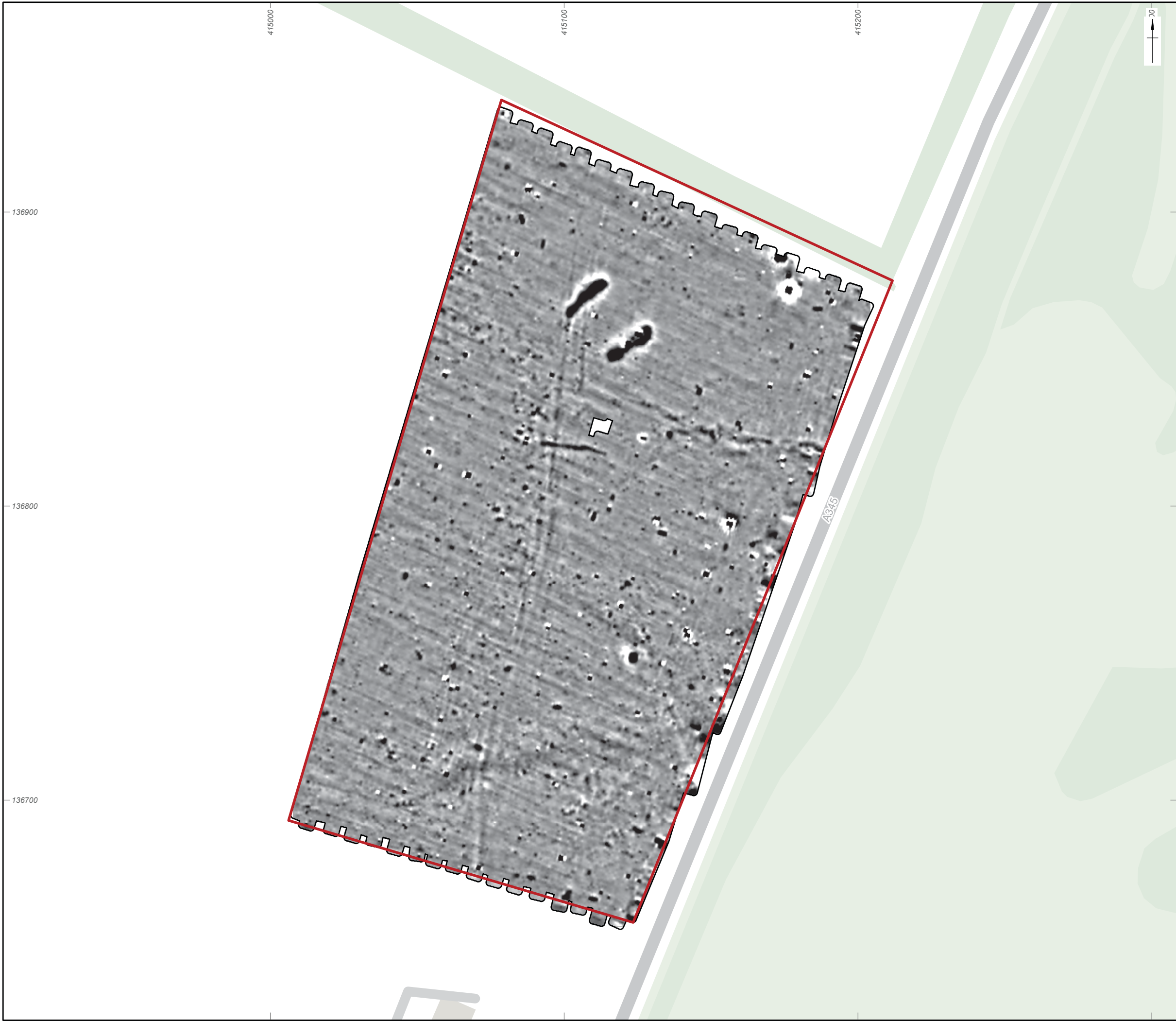
Figure 2: Gradiometer survey results: greyscale plots (-2nT to 3nT)
