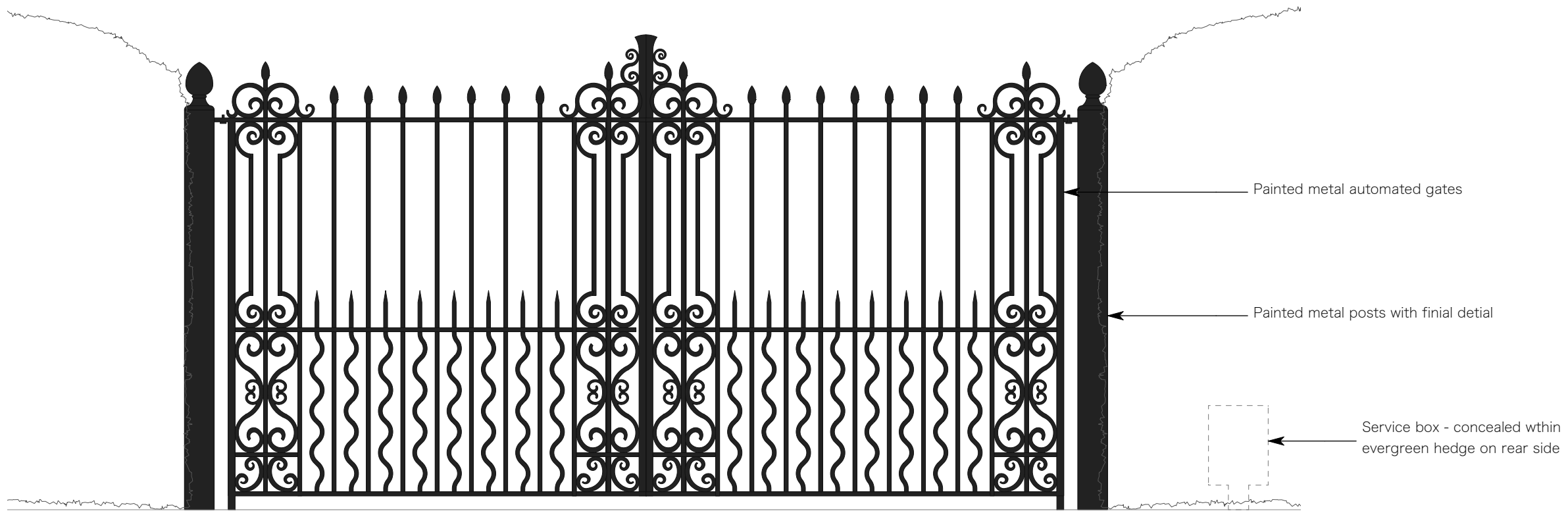
1 NORTHERN ENTRANCE GATES - EXTERNAL VIEW Scale: 1:25
