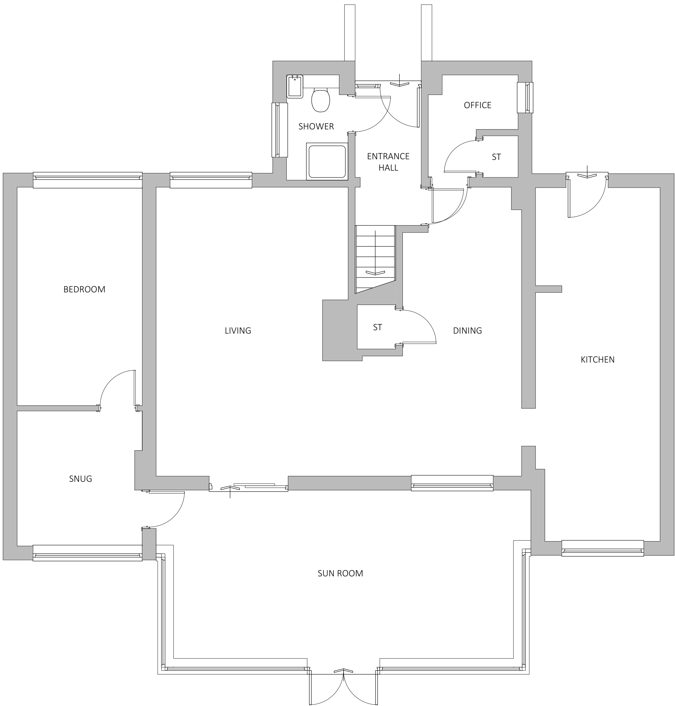
Existing Ground Floor Plan - Scale 1:50
