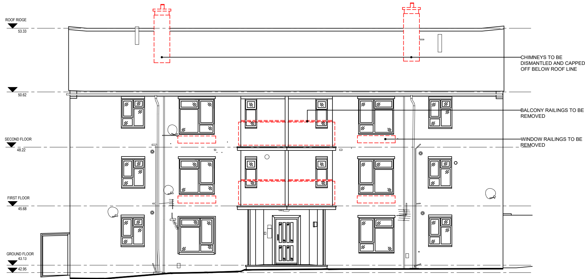
1 EXISTING - SOUTH WEST ELEVATION A/001 SCALE 1:100
