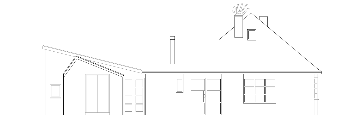
Proposed South West Elevations 2016, with decorative chimney pot installed above stack in 2022
