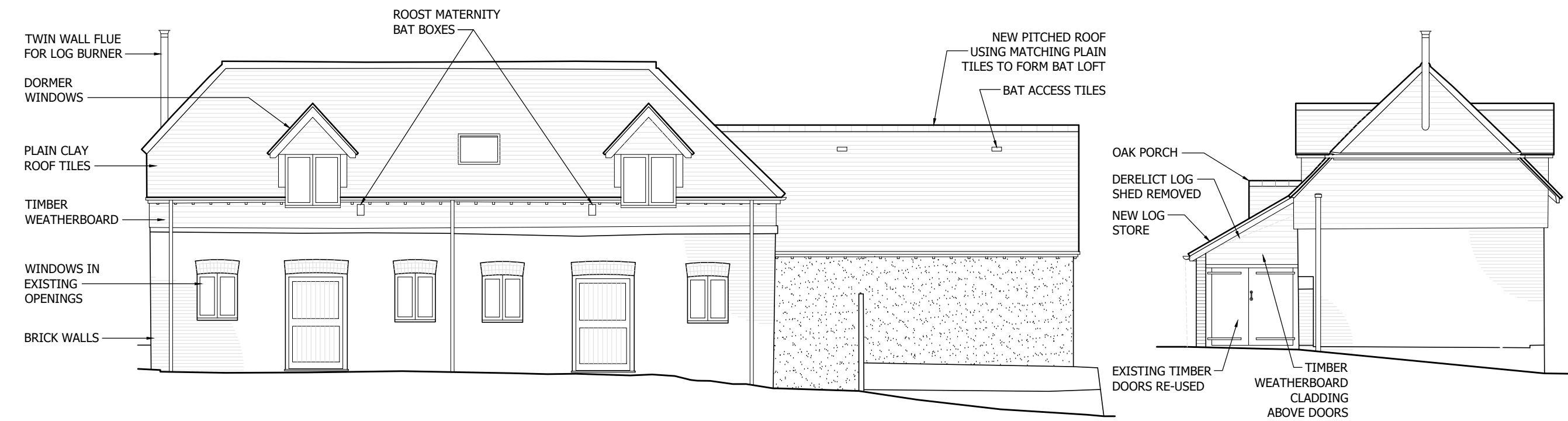
REAR ELEVATION (SOUTH-EAST) 1:100 @ A1
