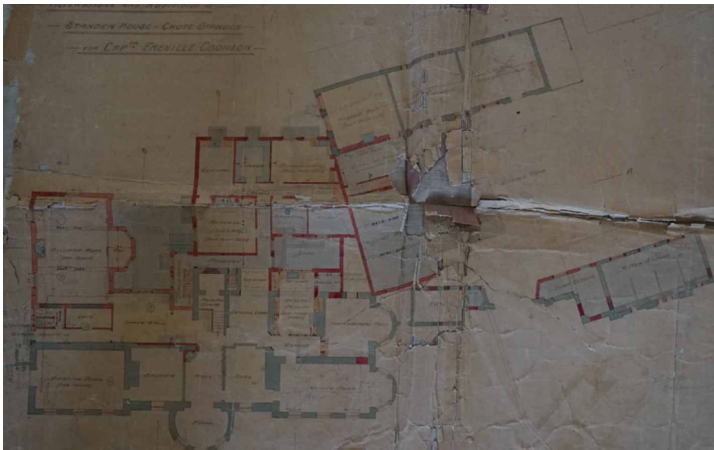
Ground floor plans Frank Verity FRIBA showing the extent of the additions. Existing fabric blue, new fabric red
