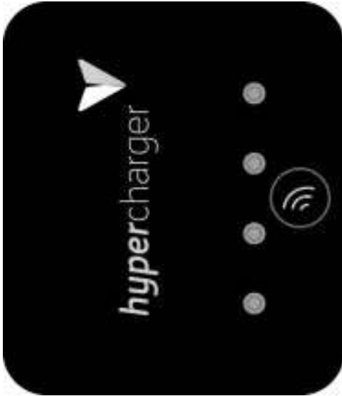
Figure 58: Position of RFID reader
