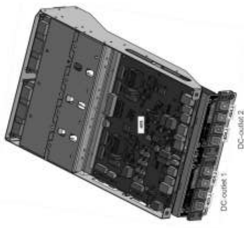
Figure 23: DC output switchgear of the HYC_150 (top view)
