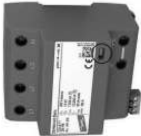
Figure 80: Check of overvoltage protection
