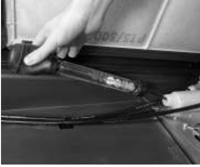
Figure 84: Check the coolant concentration using a refractometer
