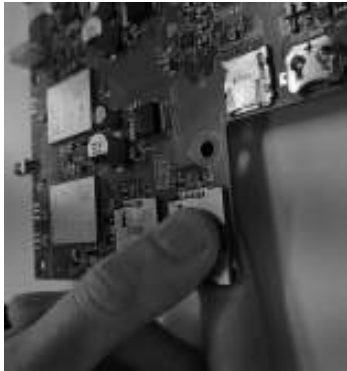
Figure 81: Compress the sim slot
