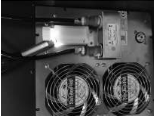
Figure 83: Checking the cooling liquid level
