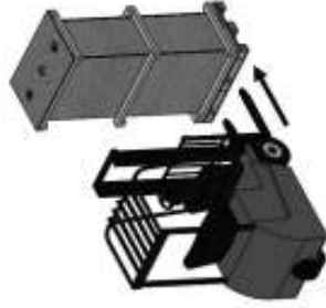
Figure 36: Vertical transport with pallet truck or forklift
