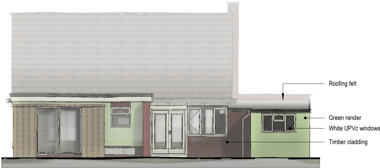
Existing Rear Elevation 1 : 100
