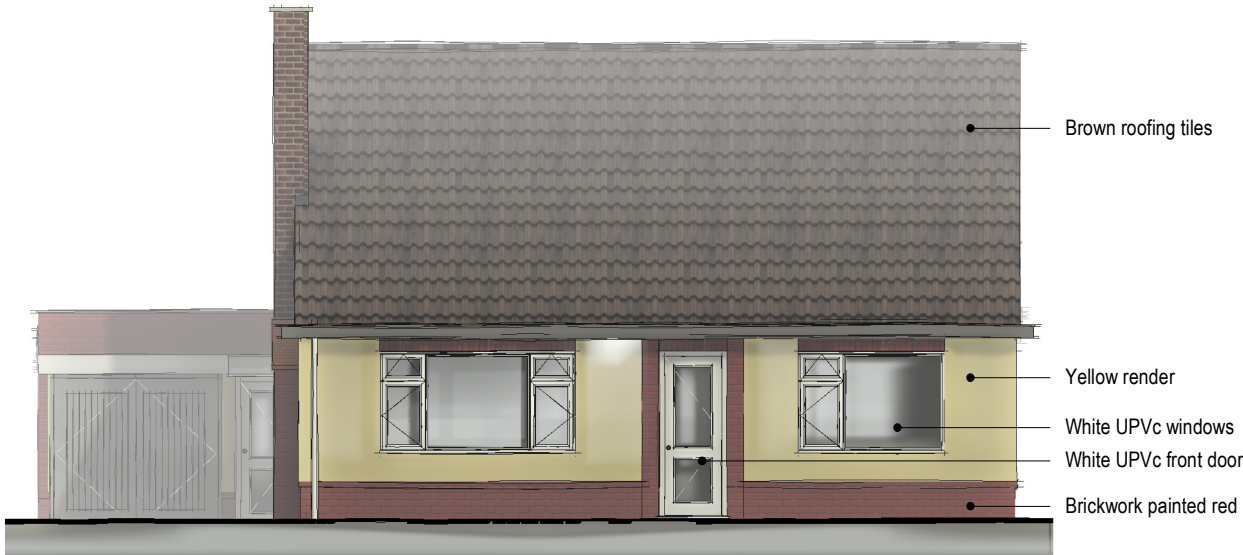
Existing Front Elevation 1 : 100
