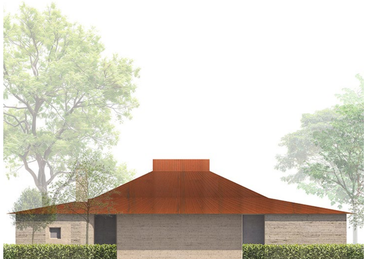
South elevation of the Pavilion with thin eaves and kinked roof
