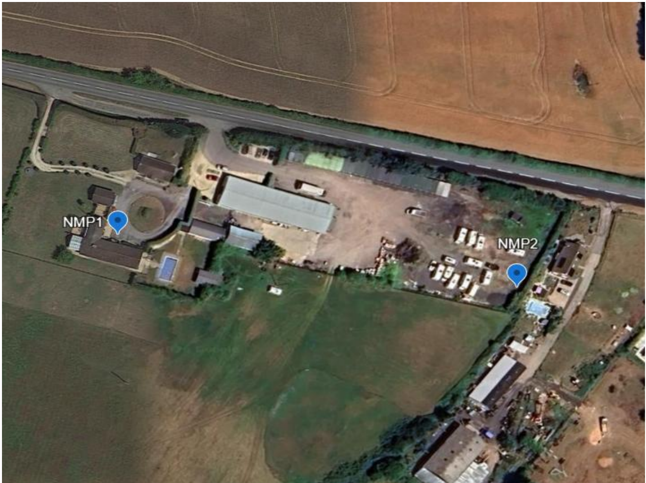
Figure 1 Noise Measurement Positions (NMP's)
