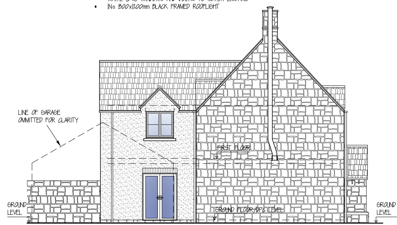
PROPOSED NORTH EAST (SIDE) ELEVATION & SITE SECTION
