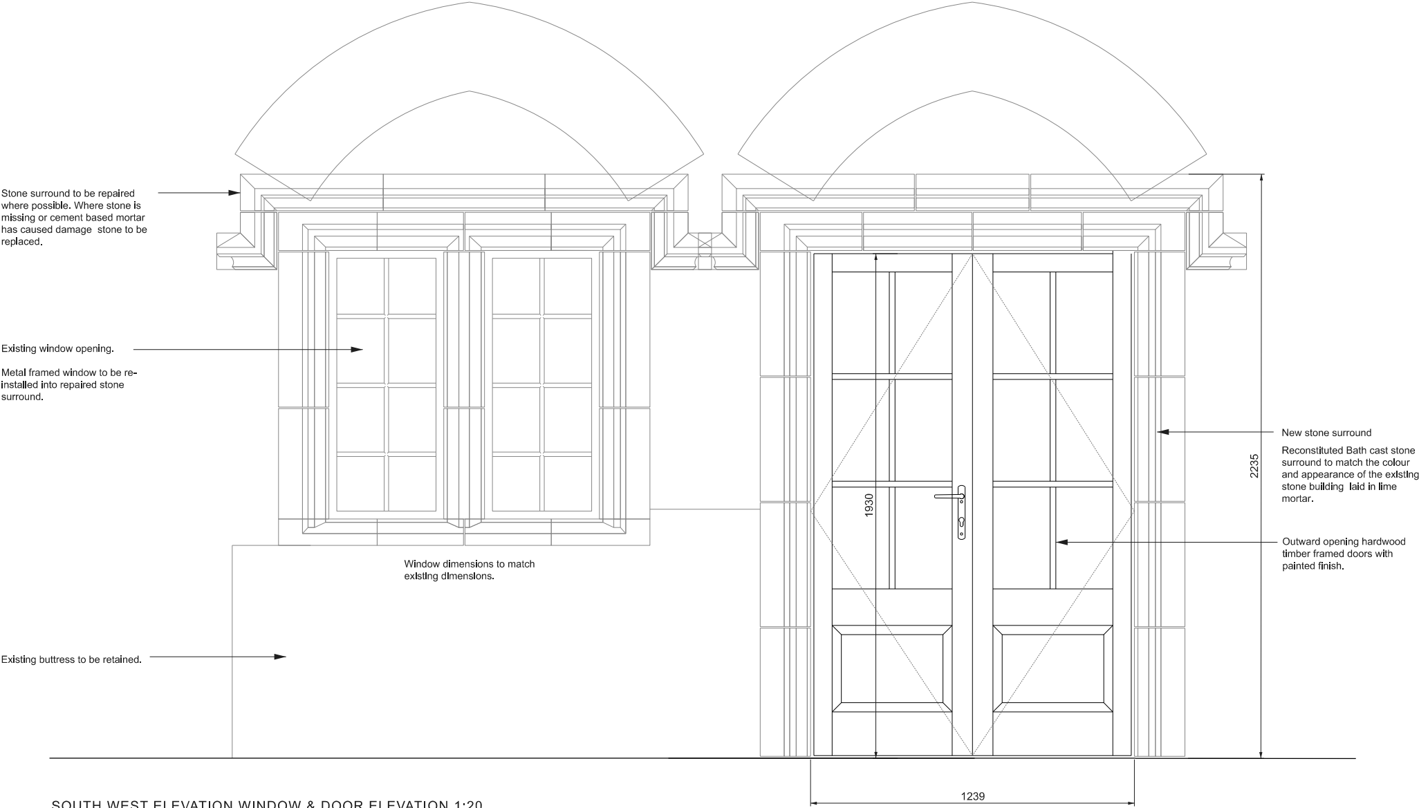
SOUTH WEST ELEVATION WINDOW & DOOR ELEVATION 1:20
