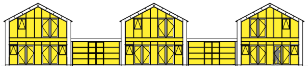
SW elevation highlighting the intended extent of fenestration
