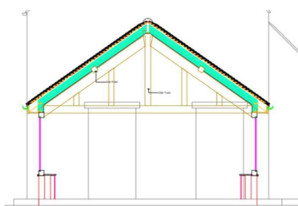
The approved Oak Truss Detail
